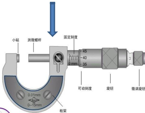
This microcalliper is used to measure the thickness of plastic tape and plastic bags, if you have no idea of the method how to use it, you can click the left button to learn.
