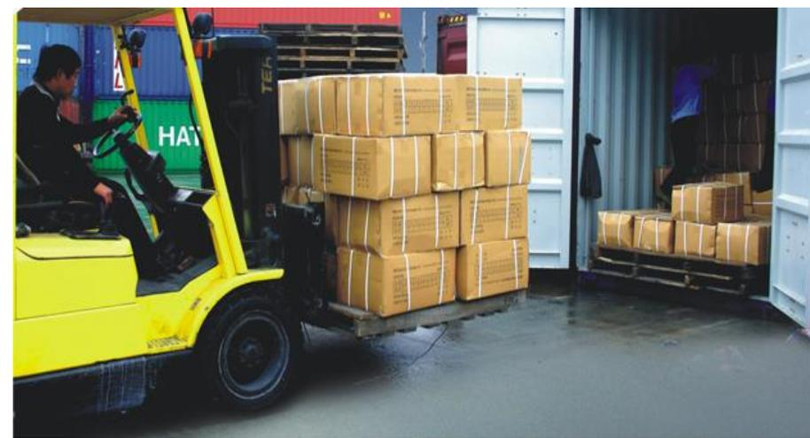
The above pictures is a 20" container,the outer size of it is 20x8x8feet 6inch,inner capacity is 5.69x2.13x2.18m,Gross weight of the cargo inside normally 17.5ton,volume is about 24-26CBM.
